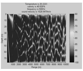
Fig. 7- The fifth graph of  $72^{nd}$  station with water characteristic full depth, source frequency is 500 Hz.
