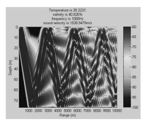
Fig.3- The fifth graph of  $72^{nd}$  station with water characteristic of full depth, source frequency is 1000~Hz.
