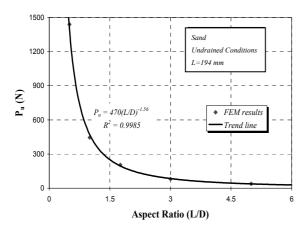
Fig.18- Aspect ratio effects (L remains constant) on pull-out capacity of suction caissons in sand under undrained conditions.
