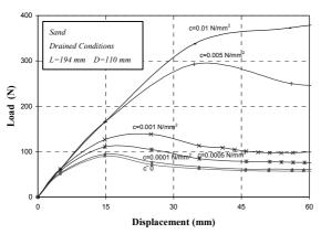
Fig.8- Soil cohesion effects on numerical pullout responses of suction caissons in sand under drained conditions.
