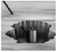
Fig.1- Schematic view of a suction anchor pile [1]
