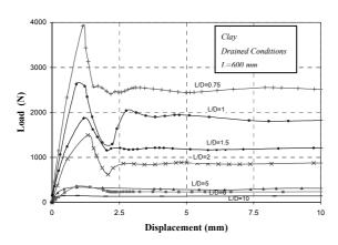
Fig.16- Aspect ratio effects (*L* remains constant) on numerical pull-out responses of suction caissons in clay under drained conditions (models are based on test data from El-Gharbawy and Olson [6])
