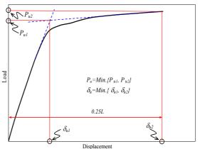
Fig.4- Pull-out capacity with suction caissons performing post ultimate softening behavior (top) and post ultimate hardening behavior (bottom), as defined in the current study.
