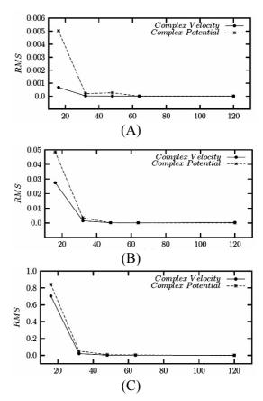
Fig. 4- RMS of pressure coefficient,  $C_p$ , for an ellipse; (A) c=0.3, (B) c=0.5, (C) c=0.7
