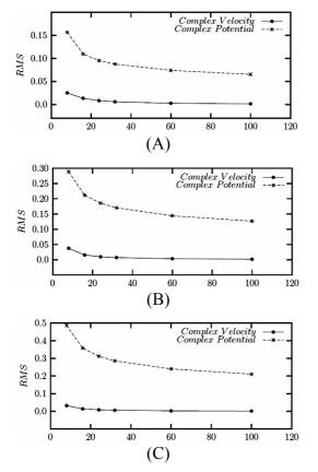
Fig. 4- RMS of pressure coefficient,  $C_p$ , for Joukowski airfoil; (A) c=0.3, (B) c=0.5, (C) c=0.7
