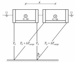
Fig. 2- Displacement in surge degree of freedom
