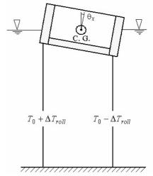
Fig. 3- Displacement in roll degree of freedom
