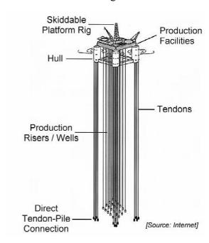
Fig. 1- TLP configuration and components
