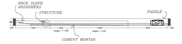
Fig. 2 - Cross section of wave flume
