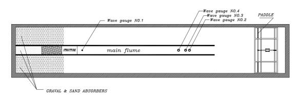
Fig. 1 - Plan view of wave flume and setup of wave height meters
