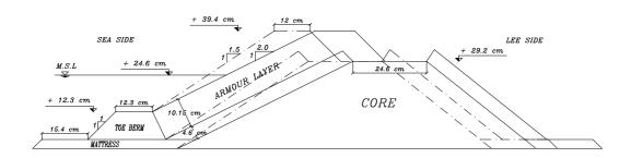
Fig. 3 - Tested Cross sections (slope = 1:1.5 & 1:2)
