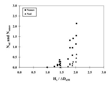
Fig. 4 -  $N_{od}$  and  $N_{omov}$  versus the stability number (cota = 1.5)
