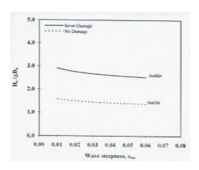
Fig 6- The stability number versus the wave steepness for mean period
