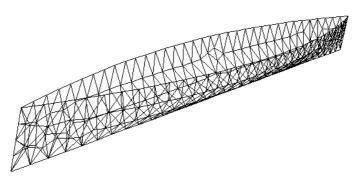
Figure 2- Triangular elements on hull form
