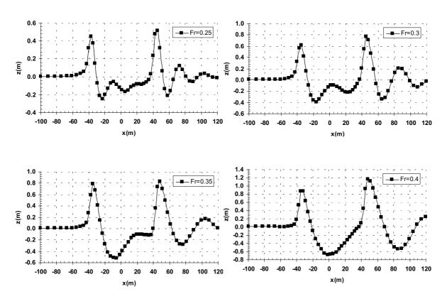
Figure 7- Wave profile on centerline
