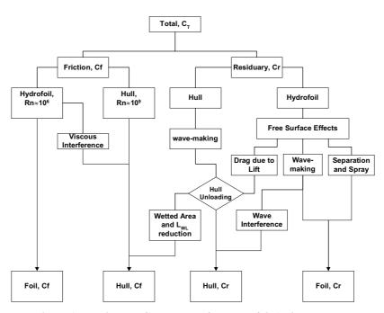
Figure 1 - Resistance Components for Hydrofoil Assisted Vessels
