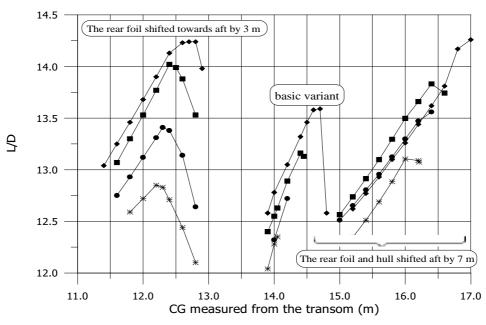
Figure 9 - The L/D ratio versus the position of the center of gravity for three cases . The wave resistance is taken into account. Diamonds- 170 t, bars- 180 t, circles- 190 t, stars- 200 t
