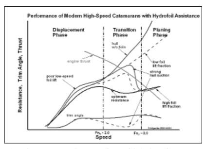
Figure 2 - Hydrodynamic Phases of hydrofoil Assisted Catamarans
