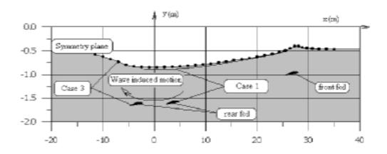
gure 11- The mutual positions of the rear foil and the wave surface at 40 knots.
