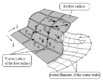
Figure 4 - Vortex Lattice of the free surface and vortex wake behind the hydrofoil
