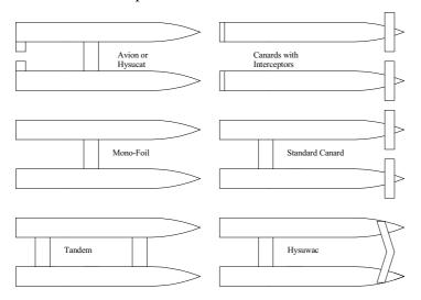
Figure 3 - Foil Configurations for Hydrofoil Assisted Catamarans
