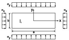
Fig. 3- Simply supported plate under thrust
