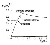
Fig. 4- Average stress-average strain relationship of a square plate (1000x1000x15.5 mm) under thrust
