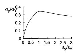
Fig. 11- Average stress-average strain relationship of a rectangular plate (2400x835x15 mm) under transverse thrust
