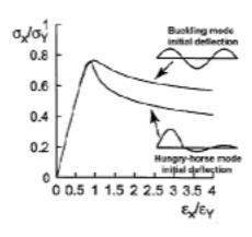
Fig. 9- Average stress-average strain relationship of a rectangular plate (2400x835x15 mm) under longitudinal thrust
