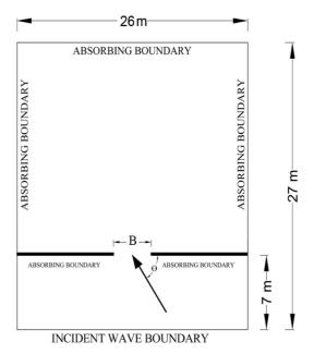
Fig. 1-The layout of computational domain.
