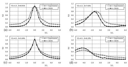
Fig. 3- Comparison of the computed and measured diffraction coefficients for unidirectional irregular waves ( $\gamma=1$ ,  $s=\infty$ ), B=3.92 m (B/L=2)
