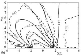
Fig. 2- Comparison of the computed and measured diffraction coefficient contours for B=7.85 m, B/L=4, multi-directional irregular waves, s=6,  $\theta_0=90^\circ$  and  $45^\circ$ . (solid line: numerical, dashed line: experimental)
