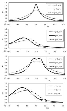
Fig. 9- Diffraction coefficients at section Y/L=3 for different waves: (a) B=3.92 m (B/L=2),  $\theta 0=90^{\circ}$ ; (b) B=3.92 m (B/L=2),  $\theta 0=45^{\circ}$ ; (c) B=7.85 m (B/L=4),  $\theta 0=90^{\circ}$ ; (d)  $B=7,85 \text{ m } (B/L=4), \theta 0=45^{\circ}$
