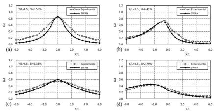
Fig. 5- Comparison of the computed and measured diffraction coefficients for irregular waves ( $\gamma$ =4, s=6), B=3.92 m (B/L=2)
