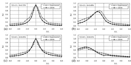
Fig. 4- Comparison of the computed and measured diffraction coefficients for unidirectional irregular waves ( $\gamma$ =4, s= $\infty$ ), B=3.92 m (B/L=2)
