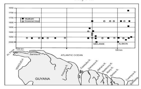
Figure 2- Representation of mudbanks along the Guyana coast Data source: field work, and [11]
