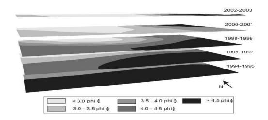
Figure 5- TIN representation of temporal variations in grain size of Melanie mudbank
